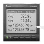
DPM-C530: dot matrix LCD for high recognition display, better than segment LCD display
